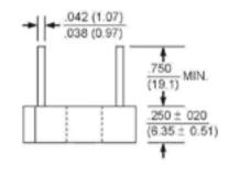
Polarity shown on side of case; positive lead by beveled corner.
