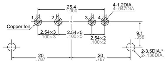
\* There 2 holes are not necessary when not using heat sink (AQ-HS-5A)
