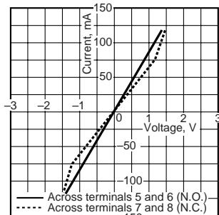
**9. Off state leakage current**
