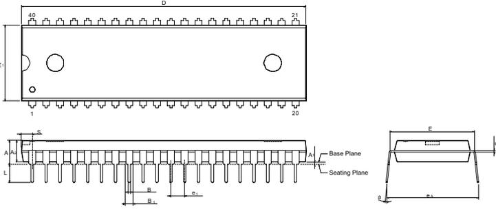
The diagram shows a top view and a side view of a 40-pin DIP package. The top view includes dimensions for length (D), width (E), and pin spacing (A, A<sub>1</sub>, A<sub>2</sub>). The side view shows the package height (E), lead length (L), and lead thickness (S). The base and seating planes are also indicated.
