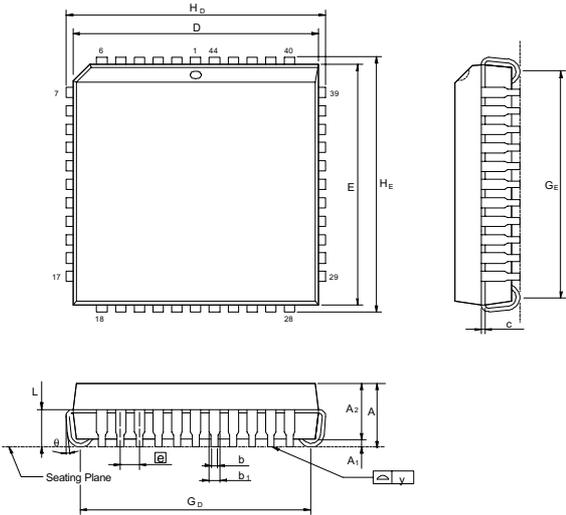
The diagram shows a top view and a side view of a 44-pin PLCC package. The top view includes dimensions for length (H<sub>D</sub>, D), width (H<sub>E</sub>, E), and pin spacing (A, A<sub>1</sub>, A<sub>2</sub>, b<sub>1</sub>, b, c, D, E, G<sub>D</sub>, G<sub>E</sub>). The side view shows the package height (G<sub>E</sub>) and lead length (L). The seating plane is also indicated.
